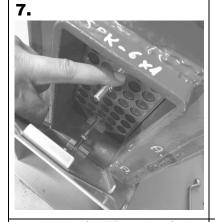
...and add the side "B" cover by using the second bold and secure cover with a nut.
