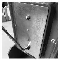
Tighten the nuts evenly until the cover side "A" & "B" are flush to frame.
