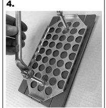
If needed, adjust the distance to 57mm.
