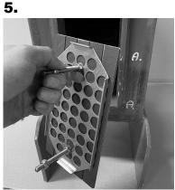
The side "A" cover is inserted diagonally through the GK packing frame ...
