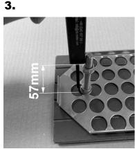
The distance between the nuts must be 57mm (Frame depth T=60mm).
