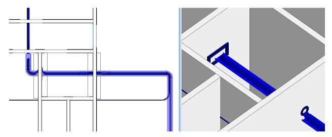
h. In case Transits are used to handle only a single cable, the 3D cable visualization will use these single Transits. In the screenshot, you can see an example in Mid-Voltage cable in red passing Mid-Voltage Transits also in red.
