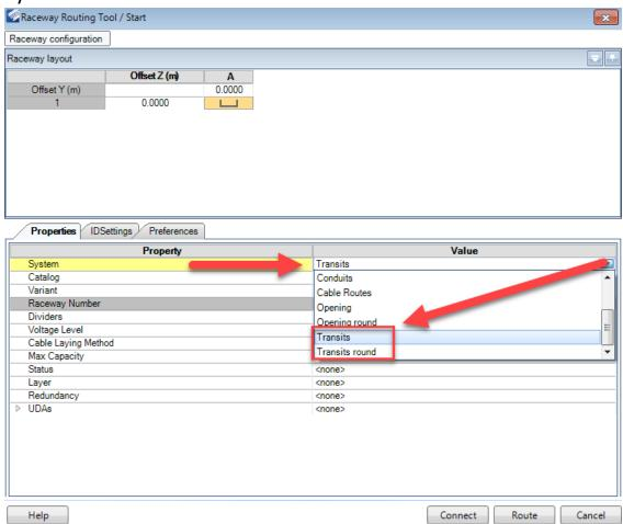
2. In the Raceway Routing Tool are two different Transit Systems, each with multiple Transit Catalogs available.
