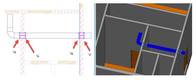
c. Next is to remove the raceway parts no longer necessary. That will create a gap between the raceways.
