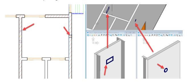
b. In the next step, the user can create required raceway systems starting or ending next to the created Transits.
