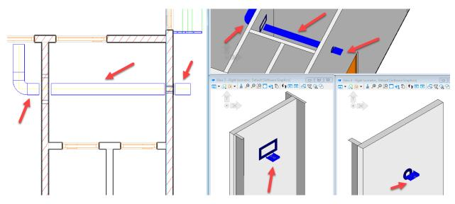
c. To enable later cable routing the raceways and Transits need to be connected. Possible usage of the BENTLEY RACEWAY AND CABLE MANAGEMENT "Generate Routing Lines" command.
