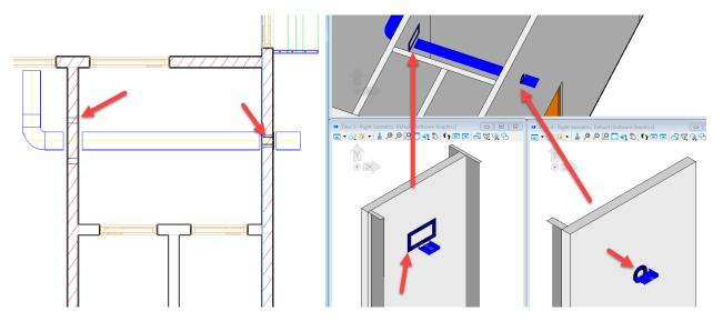
e. To enable later cable routing, using raceways and Transits, it will be necessary to connect them together using e.g. the BENTLEY RACEWAY AND CABLE MANAGEMENT "Generate Routing Lines" command.
