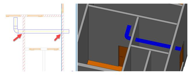
b. After the creation of the raceway systems, the user splits the created raceways using the BENTLEY RACEWAY AND CABLE MANAGEMENT "Cut Raceway" tool and cuts the raceways e.g. in front and after a wall passing.
