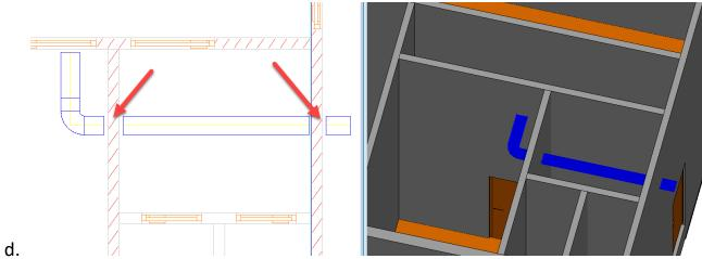
The user adds the Transit inside an opening (if it exists in the architectural drawing) or in the wall/area it will need to be.
