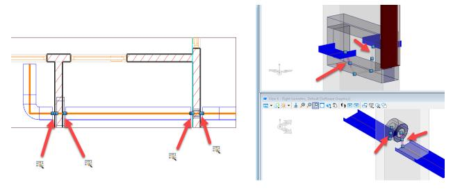
d. In BENTLEY RACEWAY AND CABLE MANAGEMENT routing file now it will be possible to manually or automatically route the cable to the related raceways and Transits.
