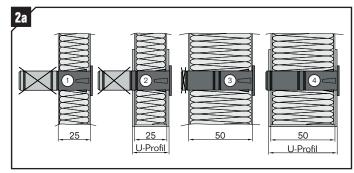
Wall installation: Adjust the length of the B15-SPC (Fig. 2) as shown in Fig. 2a. The cable entry is installed with or without a U-profile. The pre-cut notches act as a guide. The length can also be trimmed flush with the wall.
