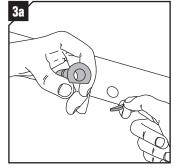
The B15-SPC cable penetration has a pre-punched flange which, when installed directly above the adjacent class division, can be adjusted without tools to allow the cable to pass through as deeply as possible.
