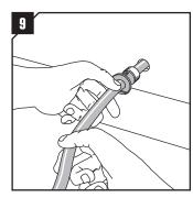
If a cable has already been laid through an opening measuring  $\emptyset$ 15mm /  $\emptyset$ 27mm, the B15-SPC cable plug can be divided by opening the inner notch and mounted lengthwise over the cable.
