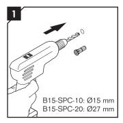
For cable penetration B15-SPC, make a perpendicular hole with the corresponding diameter (Ø15 / Ø27), if necessary remove the cutting burr.
