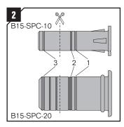
The length of the B15-SPC can be adjusted with a suitable tool prior to cable installation. A lengthwise cut is possible for already existing cables (step 6-8).
