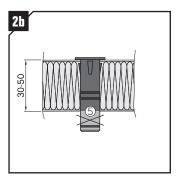
Ceiling installation: B15-SPC (Fig. 2) Adjust the length at the notches as shown in Figure 2b or install flush with the ceiling.
