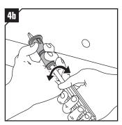
To ensure smoke gas -tightness, the B15-SPC cable penetration has a membrane inside, which is pierced using a suitable tool before the cable is installed to simplify cable installation. This can be carried out in the class division (4a) or before installation (4b)
