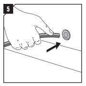
The cable is now installed from the flange side, so that the B15-SPC cable plug cannot be pushed out of the class division.
